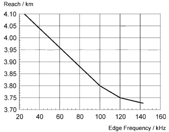
Fig. 1. Reach of the 2.048-Mb/s ADSL system dependent on the edge frequency  $f_e$  of the ADSL signal (0.4-mm wire, 1 AsIMx).
