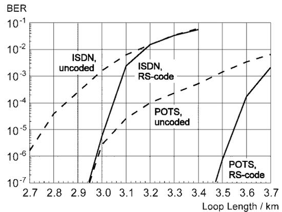
Fig. 2. Bit error ratio (BER) of uncoded and coded ADSL over POTS or ISDN (140 kHz), 2.048 Mb/s, 0.4-mm wire, 8 AsIMx.
