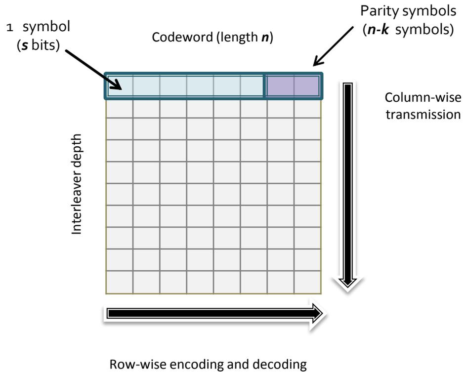
Fig. 3 10-bit interleaved system
