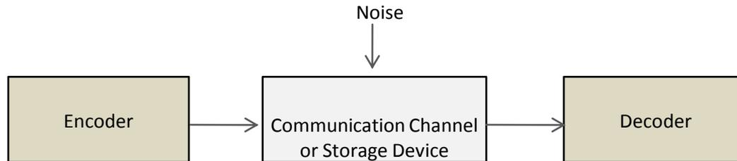
Fig 1. Typical system for encoding and decoding data
