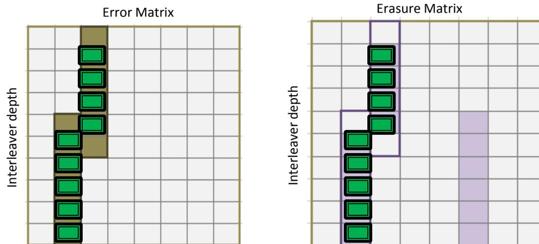
Fig. 6 10-bit interleaved system – both error and erasure matrices
