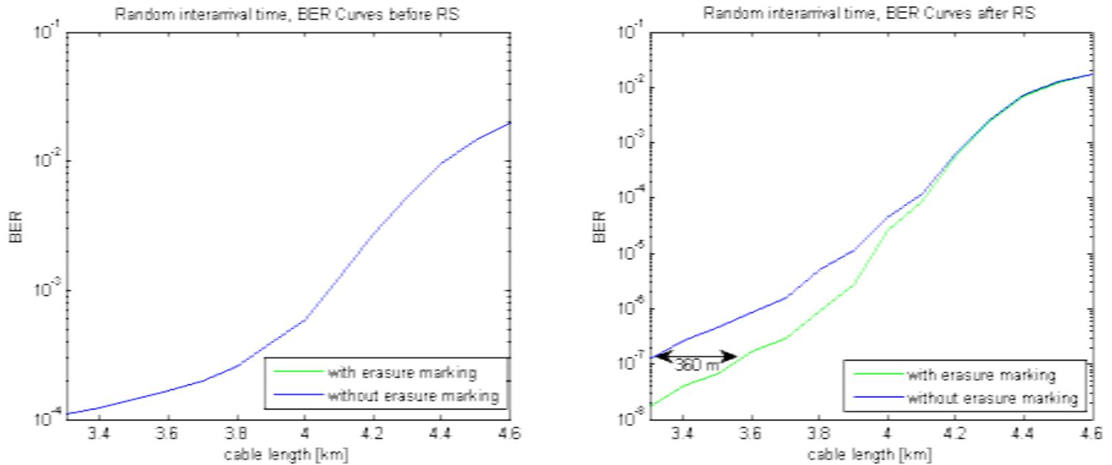
Fig. 14 BER after RS decoding in a DSL system
