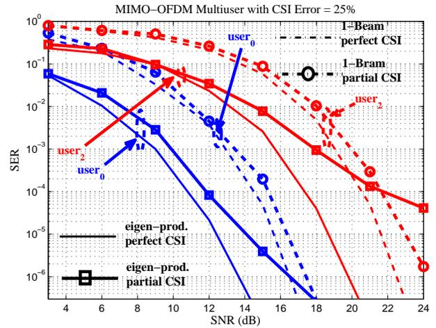
Fig. 4. Different CSI conditions for the proposed sorting schemes
