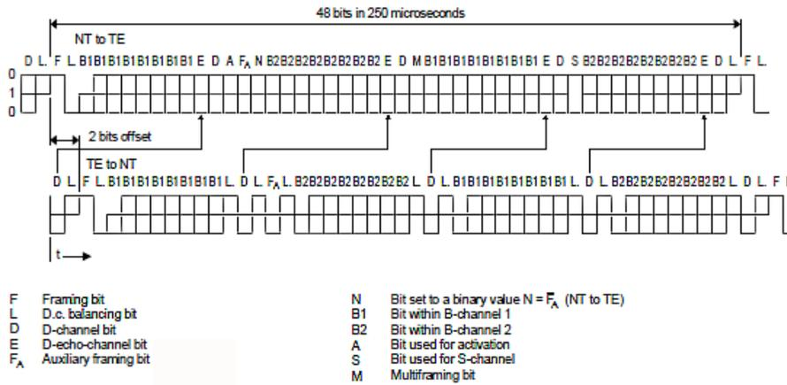
Figure 3: I.430 – Frame structure
