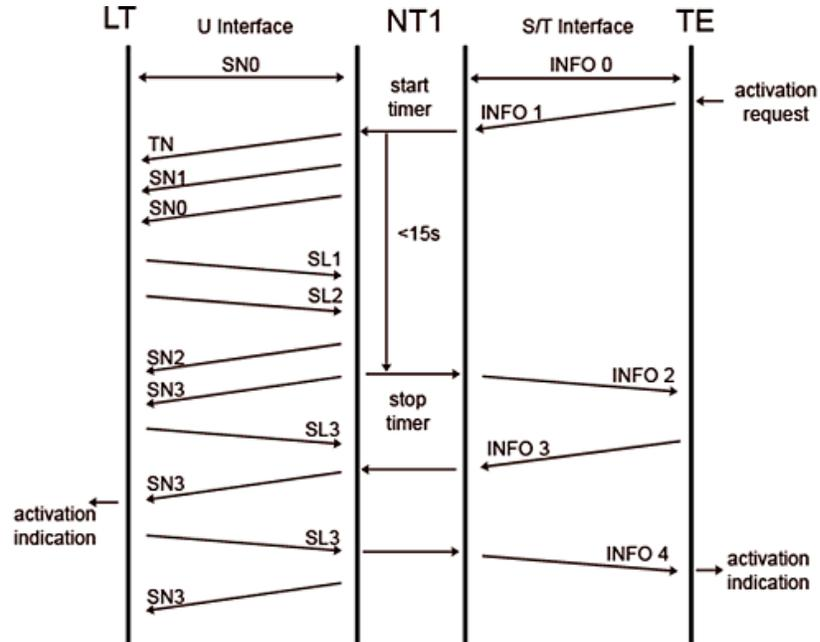
Figure 17: ETR 080 – Activation from the TE side of the 2B1Q U transmission system
