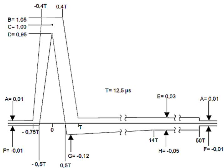
Figure 10: ETR 080 – Pulse shape for a 2B1Q transmission system
