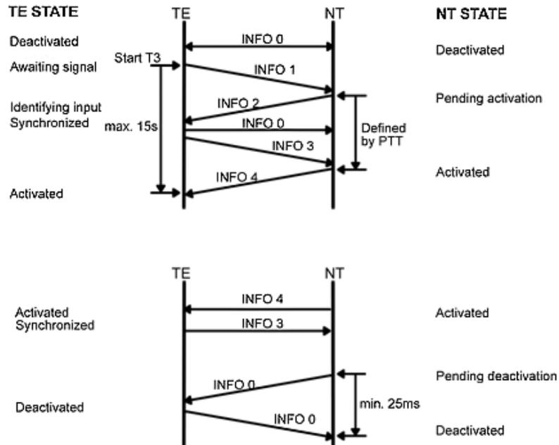
Figure 16: Activation and deactivation of the S transmission system
