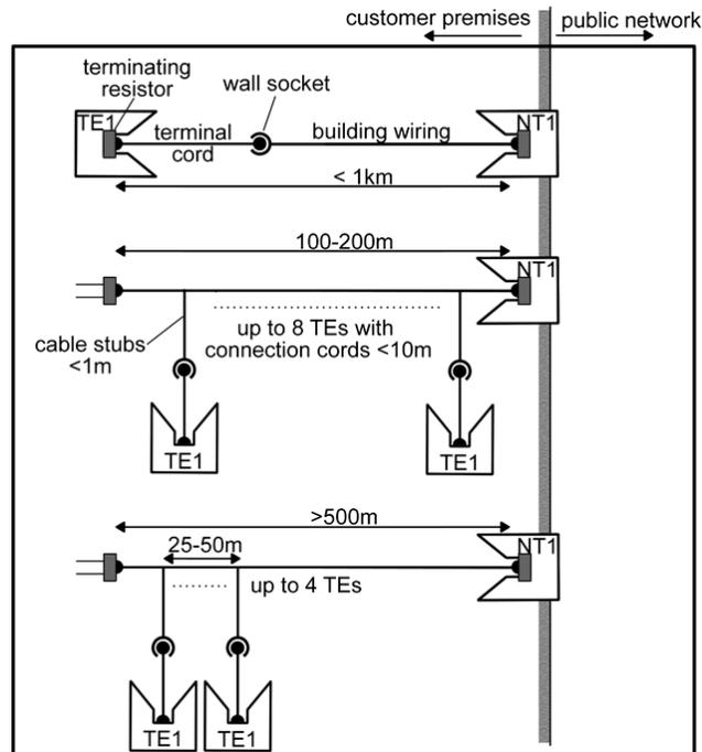
Figure 2: Wiring configurations a) Point-to-point b) short passive bus c) extended passive bus
