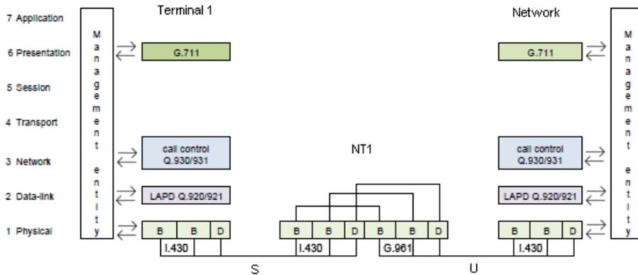
Figure 13: ISDN protocol stack
