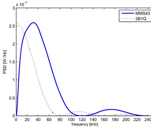
Figure 8: 2B1Q and MMS43 power spectrum densities, ISDN BRA
