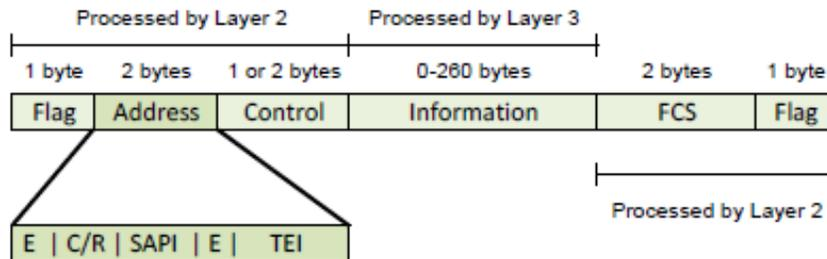
Figure 14: Q.920 LAPD frame structure
