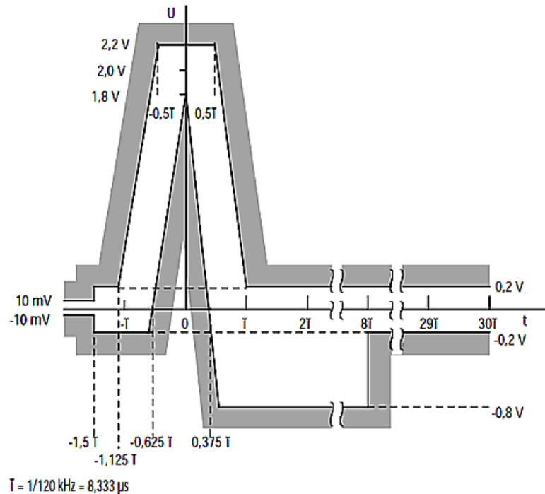
Figure 12: ETR 080 – Pulse mask for MMS43 U transmission system
