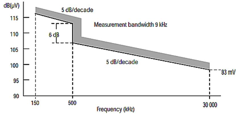
Figure 11: ETR 080 – MMS43 spectral mask
