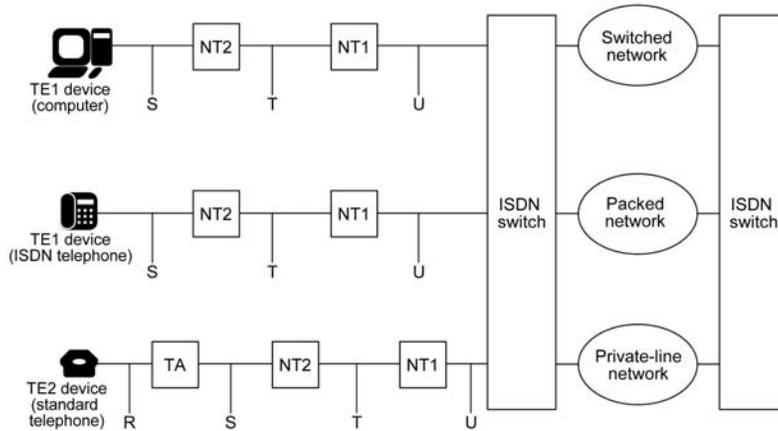
Figure 1: ISDN Subscriber loop reference model
