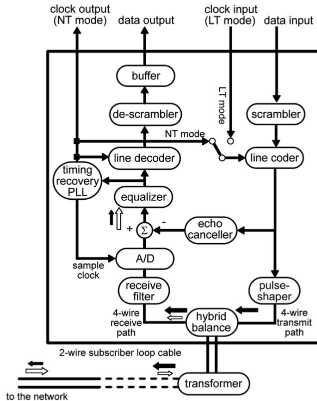
Figure 6: U transceiver - main functions
