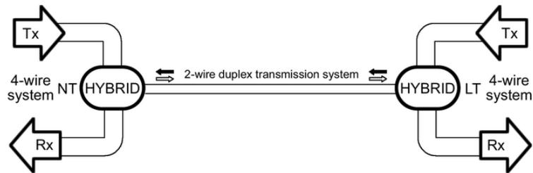
Figure 5: A typical 2-wire transmission system using a hybrid circuit
