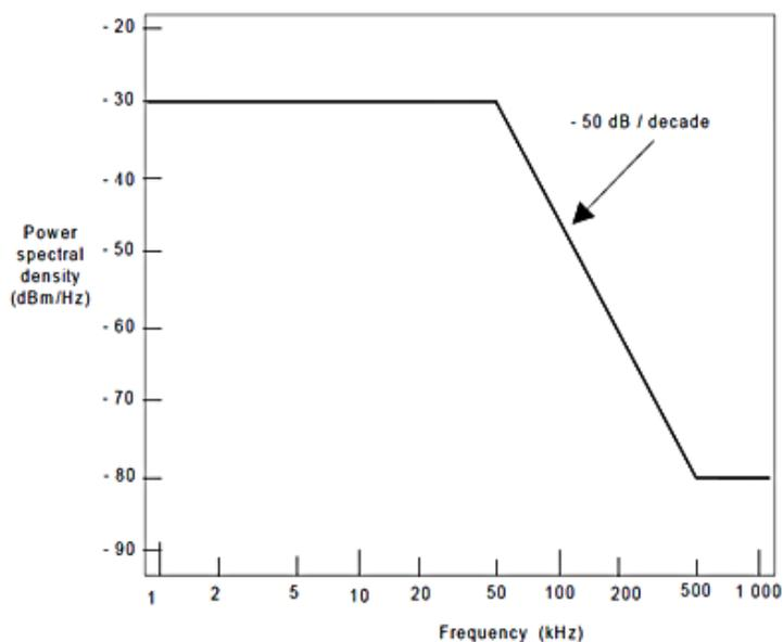
Figure 9: ETR 080 – 2B1Q spectral mask
