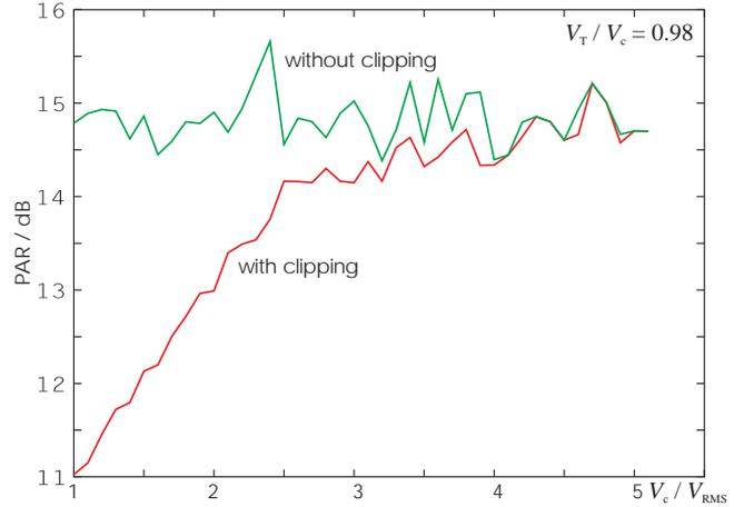
Fig. 4: PAR after filtering (rectangular) dependent on the ratio of the clipping amplitude relative to the RMS value
