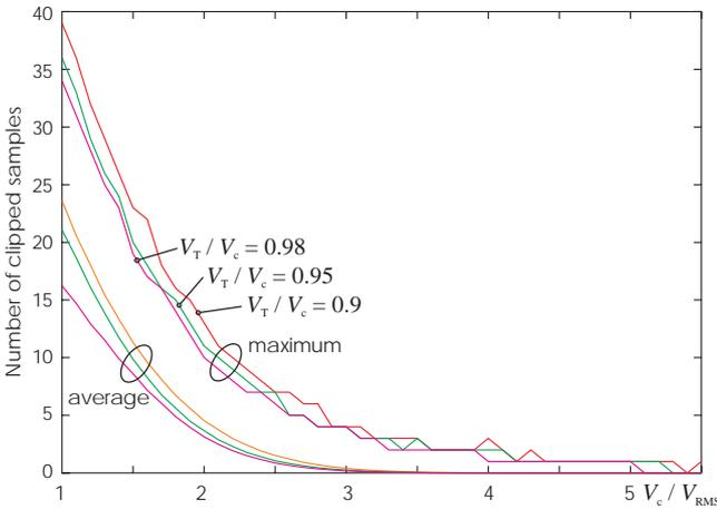
Fig. 3: Average and maximum numbers of clipped samples dependent on the ratio of the clipping amplitude relative to the RMS value
