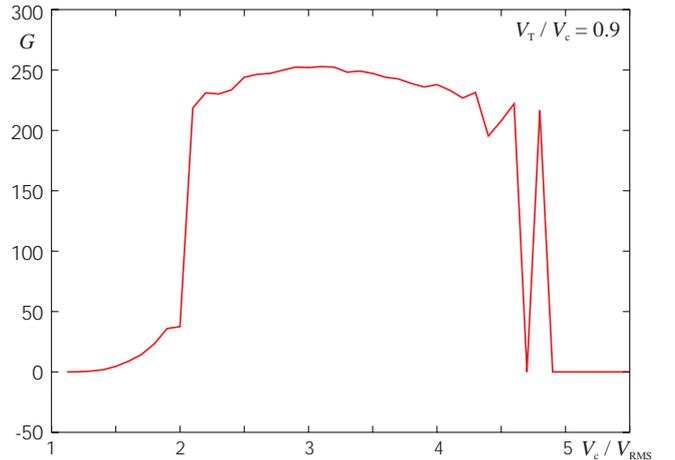
Fig. 1: Clipping-correction gain dependent on the ratio of the clipping amplitude relative to the RMS value without any filter response and without additional background noise
