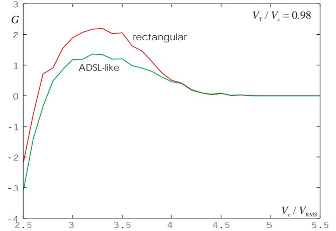
Fig. 5: Clipping-correction gain dependent on the ratio of the clipping amplitude relative to the RMS value with two different filter responses before clipping and additional background noise
