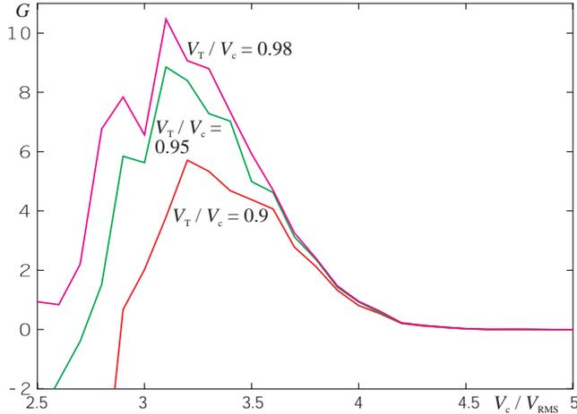
Fig. 2: Clipping-correction gain dependent on the ratio of the clipping amplitude relative to the RMS value without any filter response, but with added background noise
