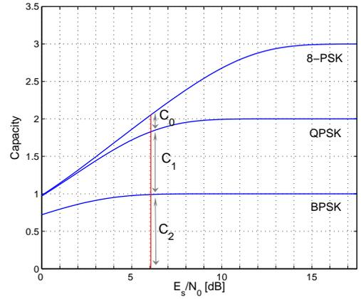
Fig. 2. Capacity curves of the partitioning levels in an 8-PSK scheme with Ungerboeck's set partitioning
