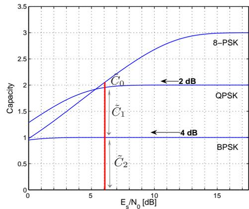
Fig. 4. Shifted capacity curves of the partitioning levels in an 8-PSK scheme with Ungerböck's set partitioning
