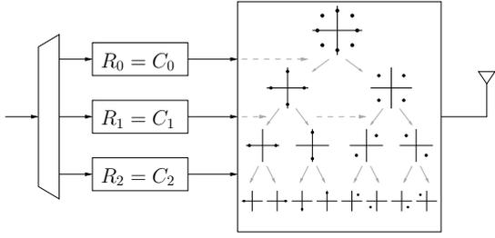
Fig. 1. Transmitter structure of an 8-PSK MLC scheme
