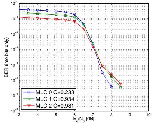
Fig. 3. Bit-error rates of the levels in an 8-PSK MLC/MSD scheme
