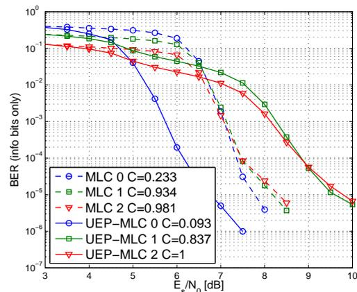
Fig. 5. Performance of an original MLC scheme and a UEP-MLC scheme with 2 dB shift in capacity curves
