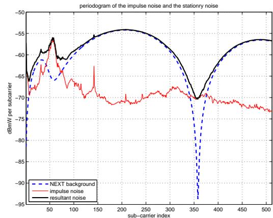
Fig. 2. Stationary background noise PSD from NEXT signals and pseudo-PSD of the impulse noise that is calculated as the average of squared FFT components of impulses
