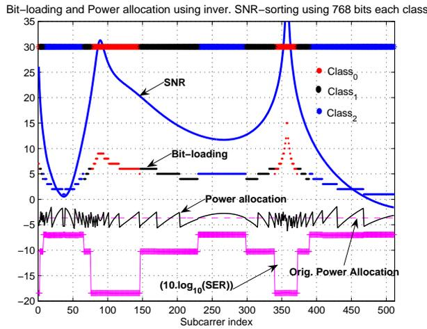
Fig. 6. Inverse SNR-sorting bit loading result for VDSL DMT with 1024 carriers using a MAR model for an Austrian 0.4-mm cable of 2 km length and T1/HDSL NEXT disturbers
