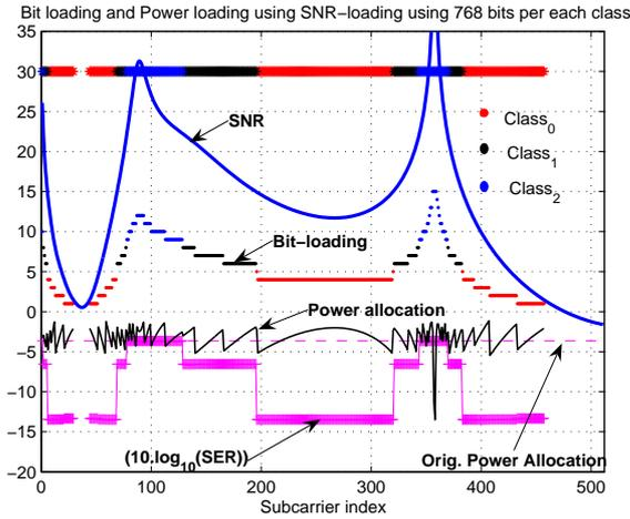
Fig. 5. SNR-sorting bit loading results for ADSL2+ DMT with 512 carriers using a MAR model for an Austrian 0.4-mm cable of 2 km length and T1/HDSL NEXT disturbers
