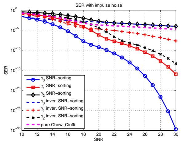
Fig. 4. The SER performance for UEP bit allocation with SNR-sorting, without SNR-sorting, and the non-UEP performance for a total target bit rate of 2304 bits per DMT symbol with 511 data carriers with real measured impulse noise as an additional disturber (bit allocation with T1/HDSL NEXT, only)
