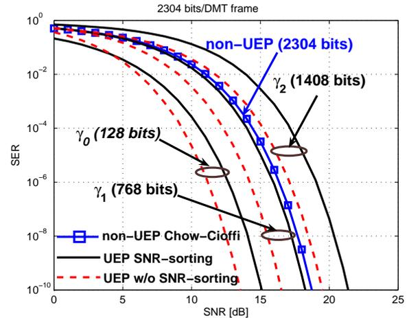
Fig. 3. The SER performance for UEP bit allocation with SNR-sorting, inverse SNR-sorting, and the non-UEP performance for a total target bit rate of 2304 bits per DMT symbol with 512 data carriers (DMT with an FFT-size of 1024) under T1/HDSL NEXT
