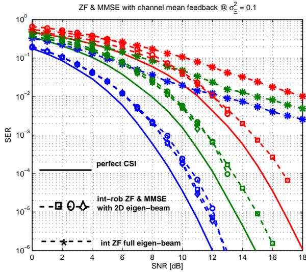
Fig. 1. Perfectly scattered channel with different beamforming equalization techniques
