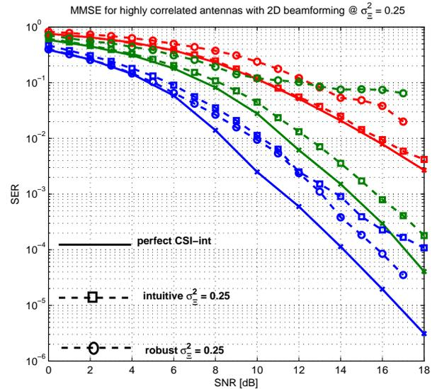
Fig. 5. Highly correlated channel with 2D beamforming at CSI errors of  $\sigma_{\Xi}^2 = 0.25$
