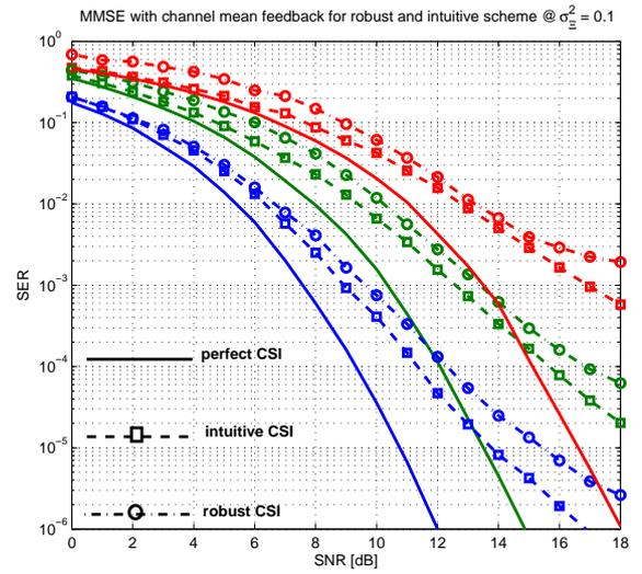
Fig. 2. Perfectly scattered channel using different sorting schemes and MMSE at a CSI error of  $\sigma_{\Xi}^2 = 0.1$
