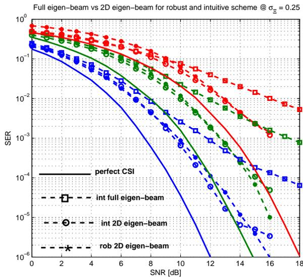
Fig. 4. Perfectly scattered channel with different beamforming and sorting schemes at CSI error of  $\sigma_{\Xi}^2 = 0.25$
