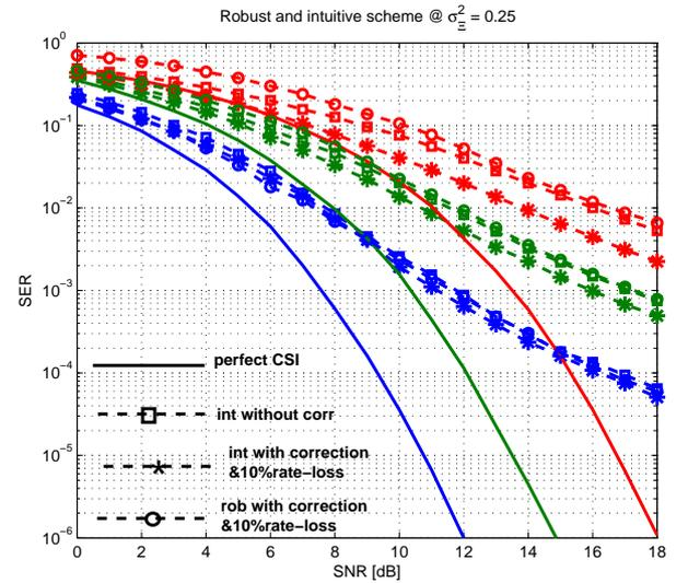
Fig. 3. Perfectly scattered channel with different sorting schemes at CSI error  $\sigma_{\Xi}^2 = 0.25$  and error compensation
