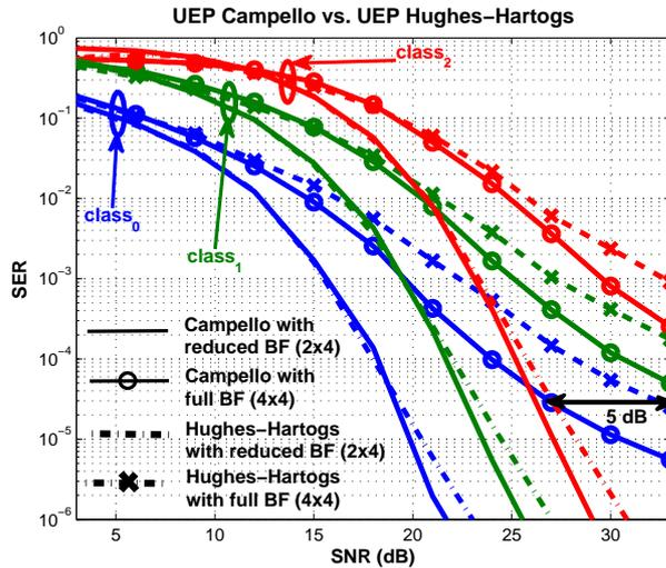
Fig. 4. A Comparison between UEP Hughes-Hartogs and UEP Campello for different beamforming in case of CSI errors.
