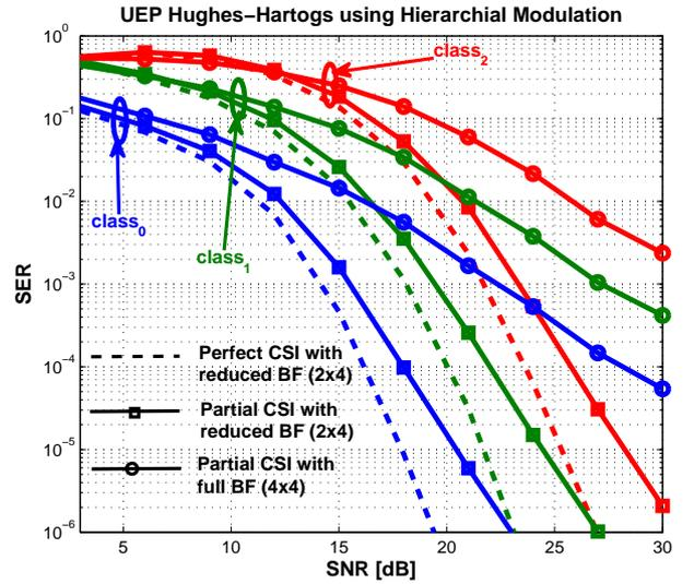
Fig. 2. Adaptive hierarchical modulation using 3 layers of UEP with 3 dB margin separation  $\gamma_j$ . The CSI errors, in case of partial feedback, is assumed to have a variance of 0.25.
