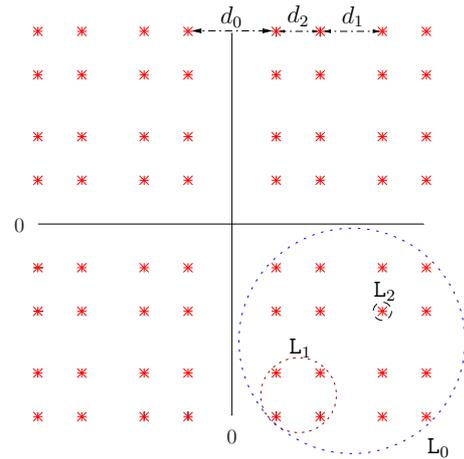
Fig. 1. Hierarchical modulation: a 4-QAM ( $L_0$ ) is embedded in a 16-QAM ( $L_1$ ) and the 16-QAM ( $L_1$ ) is, itself, embedded in a 64-QAM ( $L_2$ ) with the performance priority ratios  $d_0/d_1 = d_1/d_2 = \sqrt{2}$ .
