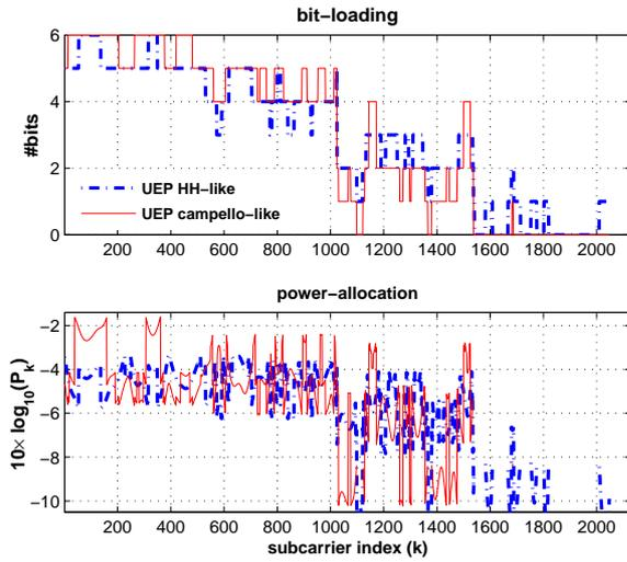
Fig. 3. Accumulated bit-loading and power allocation for 3 hierarchical layers using UEP Campello and UEP Hughes-Hartogs (HH).
