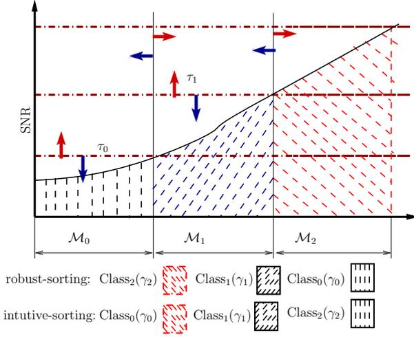
Fig. 2. SNR thresholds for three protection classes assuming Class<sub>0</sub> is the highest protected class in both schemes.
