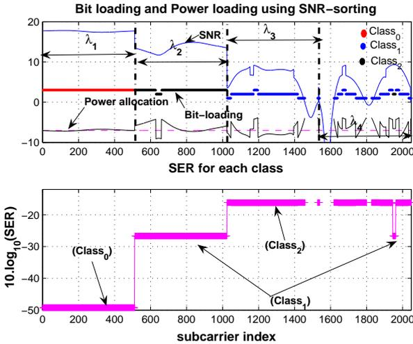
Fig. 3. UEP bit and power allocation in a 2048 subchannels MIMO-OFDM
