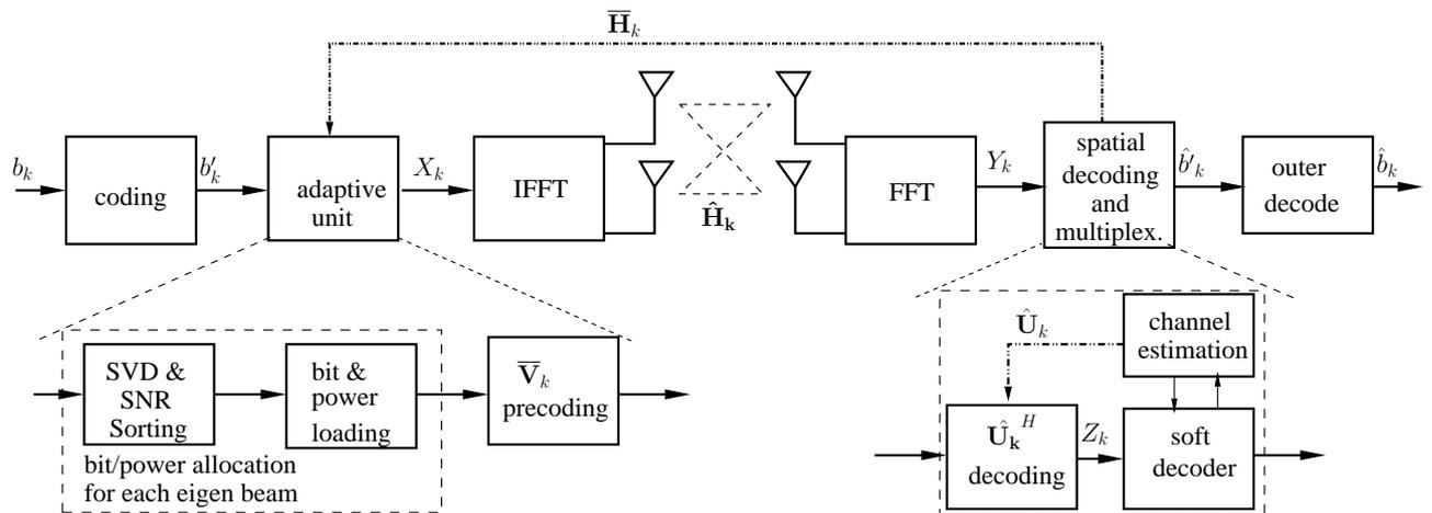
Fig. 1. MIMO UEP bit-loading
