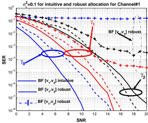
Fig. 6. Intuitive and robust allocation for the protection classes at channel feedback error of variance  $\sigma_\epsilon^2 = 0.1$
