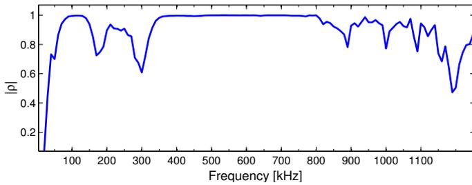
Fig. 5. Frequency dependent correlation coefficient between DM and CM for the ADSL spectral range.
