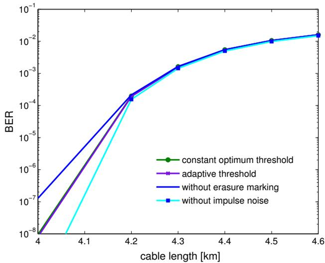
Fig. 8. Scenario #2: BER after RS decoding for the slightly impulsive environment. As expected, when the main interference source is AWGN and no other stronger interferers are present, the improvement obtained by employing the erasure scheme is not very significant.
