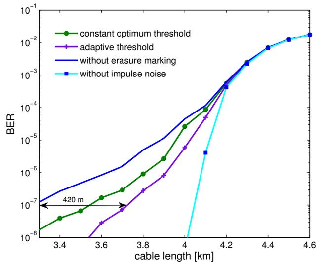
Fig. 7. Scenario #1: BER after RS decoding for the highly impulsive environment. The proposed erasure marking scheme has a significant gain when presented with a strongly impulsive case.
