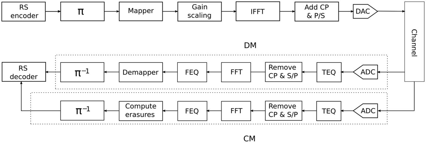
Fig. 4. Proposed system diagram. No changes are necessary at the transmitter side. At the receiver side, joint DM-CM processing is performed.
