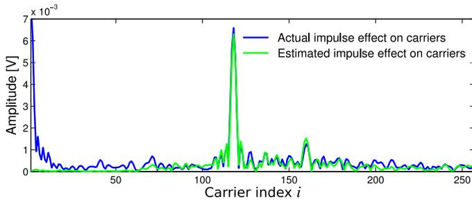
Fig. 6. Carriers corrupted by impulse noise obtained from measurements and estimated impulse noise. For this plot, one measured impulse originating from fluorescent light switching was used.
