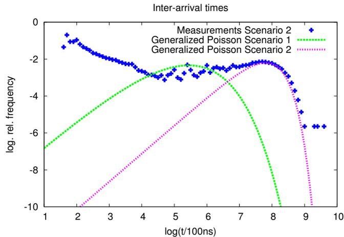
Fig. 3. Logarithmic plots of impulse inter-arrival time approximated by generalized Poisson distributions with parameters in Table I.
