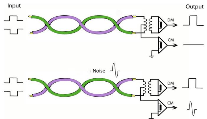
Fig. 1. DM vs. CM signaling. Here, square pulses have been used for illustrative purposes, which is not the case in practical situations. The simulation results described in Section V have been obtained by employing an Asymmetric Digital Subscriber Line (ADSL) transmission system as described in [5].
