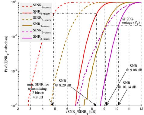
Fig. 2. Outage probability for different vSNR<sub>T</sub> and SINR<sub>T</sub> for 2, 3, and 4 users with a minimum SINR<sub>T</sub> = 4.8 dB and a maximum outage probability  $P_T = 20\%$  (80% of the subcarriers can be multiplexed)
