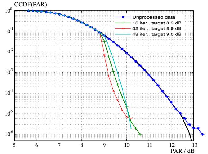
Fig. 8. CCDF of the Tone Reservation for a  $4 \times 4$  PtPt MIMO-OFDM depending on the number of iteration with joint search
