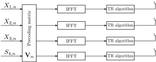
Fig. 6. Transmitter system model of MIMO-OFDM for TR algorithm
