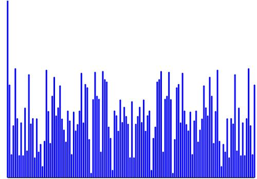
Fig. 4. Absolute values of the spiky time-domain vector used in the iterations of the Tone Reservation algorithm
