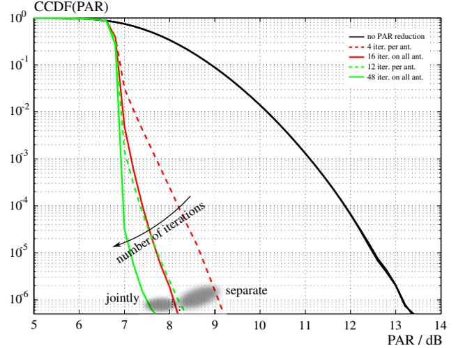
Fig. 3. CCDF of the PAR of Tone Reservation for  $4 \times 4$  multi-user broadcast with 10 % redundancy depending on the number of iterations carried out separately per antenna or with joint processing
