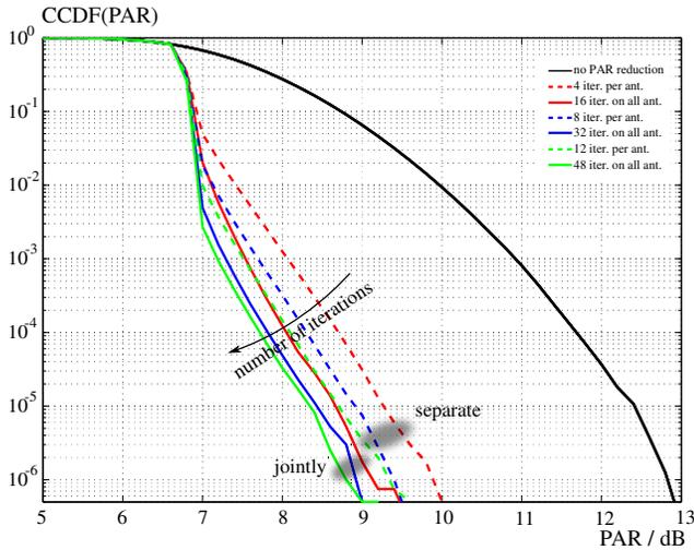
Fig. 2. CCDF of the PAR of Tone Reservation for  $4 \times 4$  multi-user broadcast with 5 % redundancy depending on the number of iterations carried out separately per antenna or with joint processing
