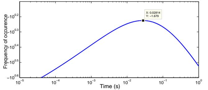
Fig. 3. Logarithmic plot of impulse inter-arrival time approximated by a generalized Poisson distribution with parameters detailed in Table I.
