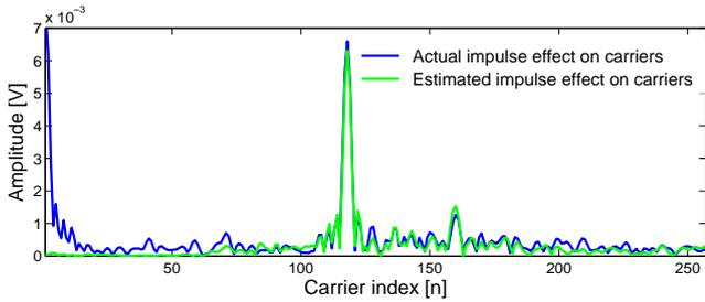
Fig. 5. Carriers corrupted by impulse noise obtained from measurements and estimated impulse noise. For this plot, one measured impulse originating from fluorescent light switching was used.
