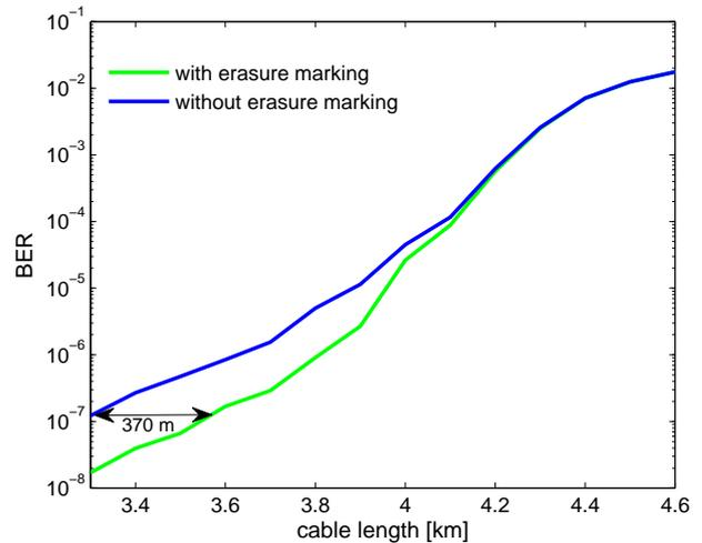
Fig. 6. BER after RS decoding when erasure marking is employed.
