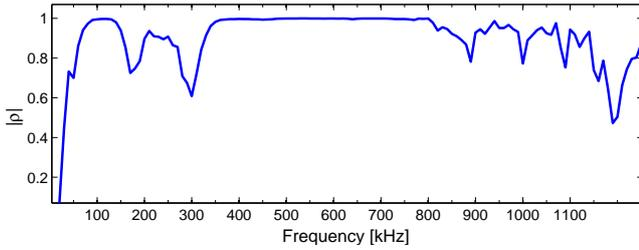
Fig. 4. Frequency dependent correlation coefficient between DM and CM for the ADSL spectral range.
