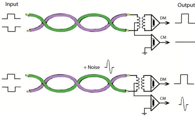
Fig. 1. DM vs. CM signaling. Here, square pulses have been used for illustrative purposes, which is not the case in practical situations. The simulation results described in Section VI have been obtained by employing an ADSL transmission system as described in [4].
