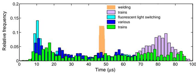
Fig. 2. Normalized histograms of impulse duration. The sets of impulses were measured in different locations in Bremen, Germany, and were caused by various sources, e.g., welding, fluorescent light switching, etc.
