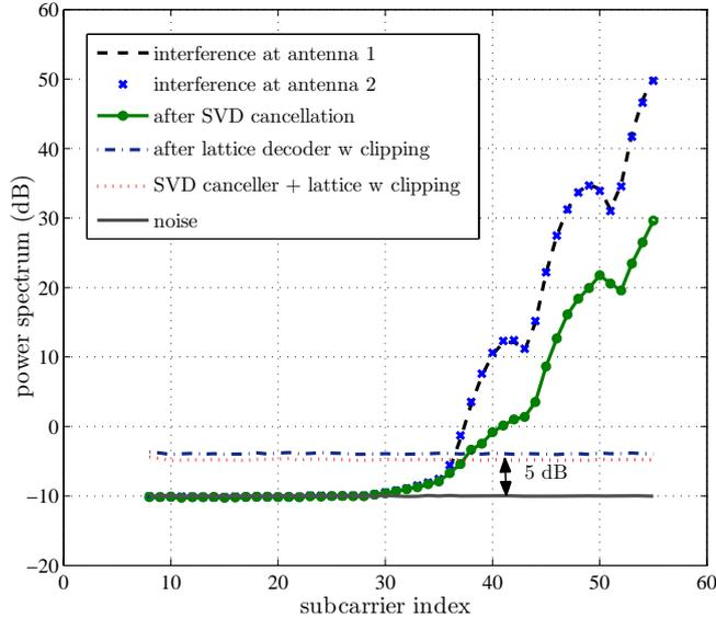
Fig. 2. Spectrum of interfering signal after the proposed SVD-based canceller at an SNR of 10 dB
