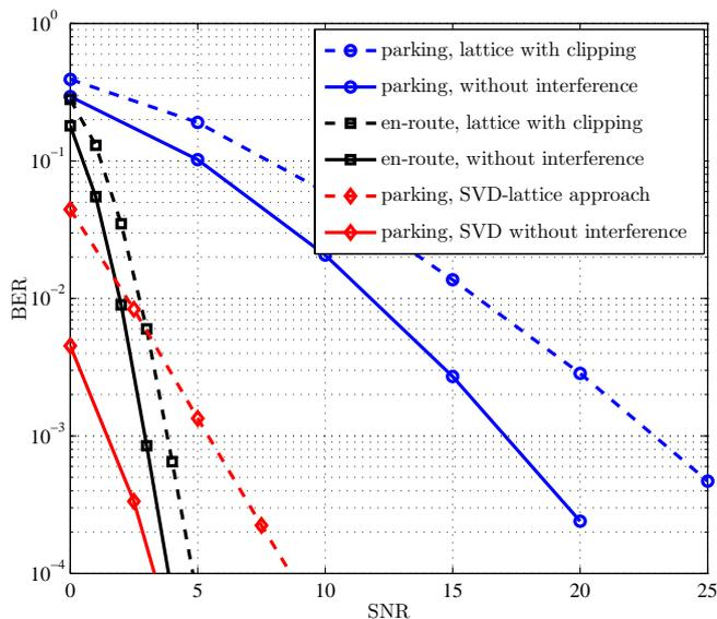
Fig. 3. BER performance over the parking and en-route channel model
