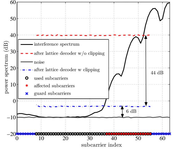
Fig. 1. Spectrum of interfering signal before and after lattice decoding at an SNR of 10 dB
