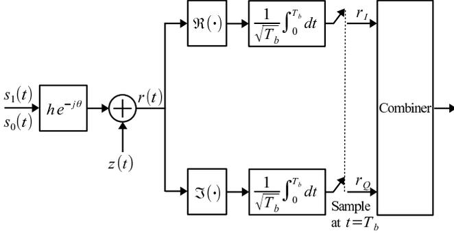
Fig. 1. A baseband model of binary signal transmission over a Rayleigh fading channel
