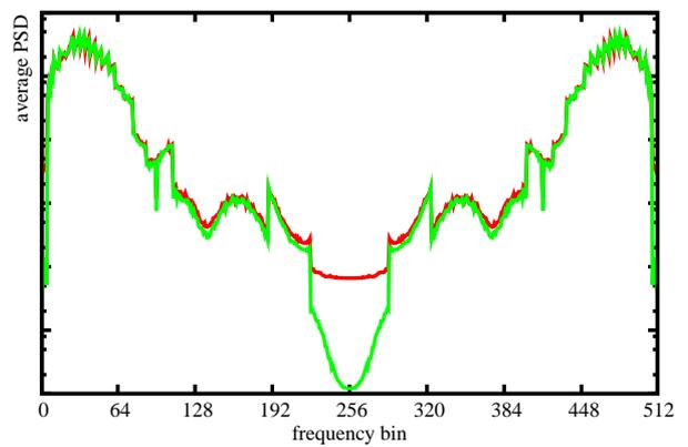
Fig. 3. Power spectral density with (green) and without (red) cyclic prefix (ADSL on a 4 km 0.4 mm loop with NEXT disturbances from 8 line multiplexers and capacity-optimizing time-domain equalization)
