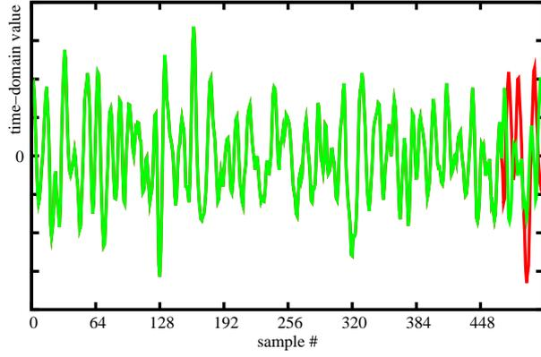
Fig. 1. ISI in case of ADSL on a 4 km 0.4 mm loop with NEXT disturbances from 8 line multiplexers and capacity-optimizing time-domain equalization
