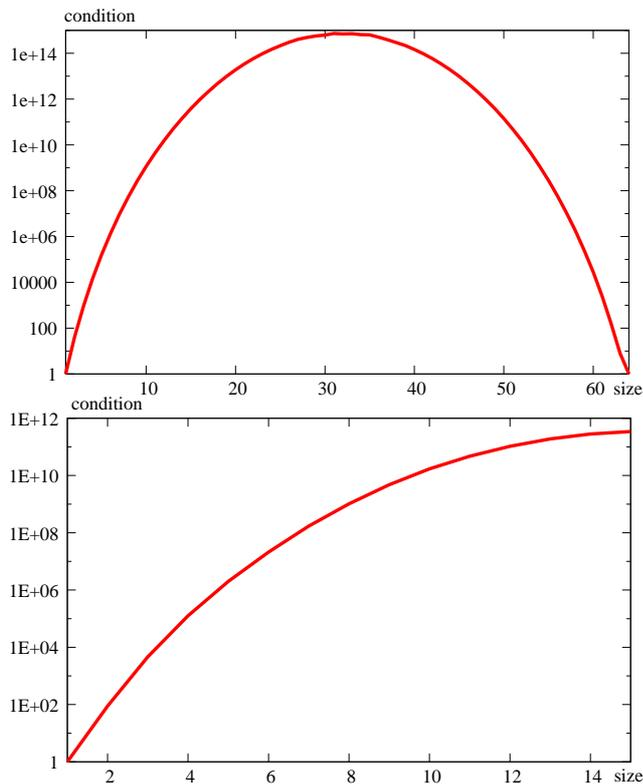
Fig. 2. Condition numbers of DFT submatrices for OFDM (upper plot) and real counterparts for DMT (lower plot) assuming the ISI to occur at the lower edge (DFT length: 64)
