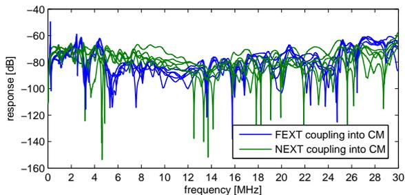
Fig. 5. NEXT and FEXT coupling functions into CM, obtained from measurements of a 0.4 mm Swiss cable of length 100 m.
