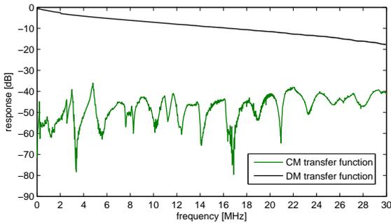
Fig. 3. DM and CM transfer functions measured on a 0.4 mm Swiss cable of length 100 m
