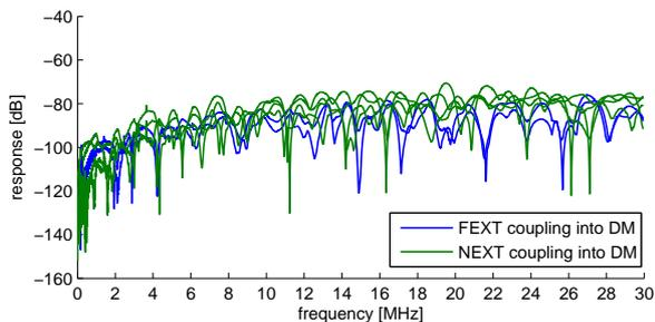
Fig. 4. NEXT and FEXT coupling functions into DM, obtained from measurements of a 0.4 mm Swiss cable of length 100 m.
