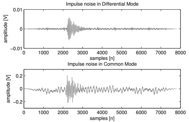
Fig. 5. Impulse noise generated from fluorescent light switching, both in DM and CM. Please note the different amplitudes of the waveforms.
