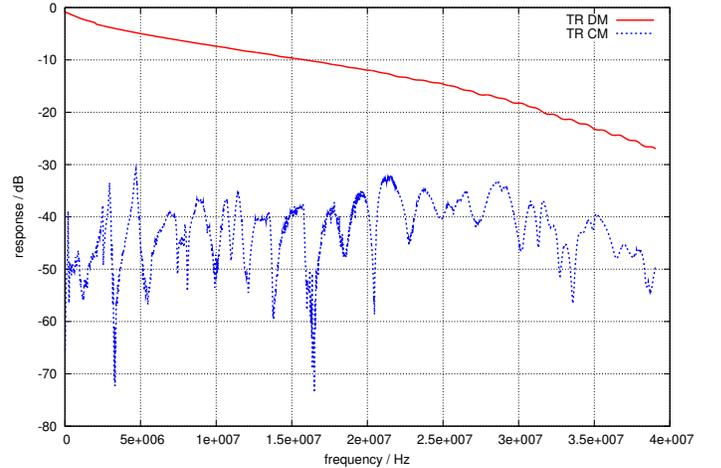
Fig. 2. Transfer functions for DM and CM obtained from measurements of a 0.4 mm Swiss cable of length 100 m
