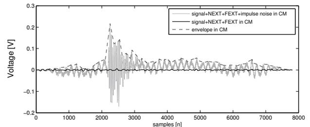
Fig. 6. Envelope of CM signal (dashed grey). The black line represents the CM coupling of the signal, along with 4 NEXT and 5 FEXT disturbers for a cable length of 3.5 km. Thin grey waveform represents the overall CM signal, including impulse noise. Impulse noise is the dominant signal in CM.
