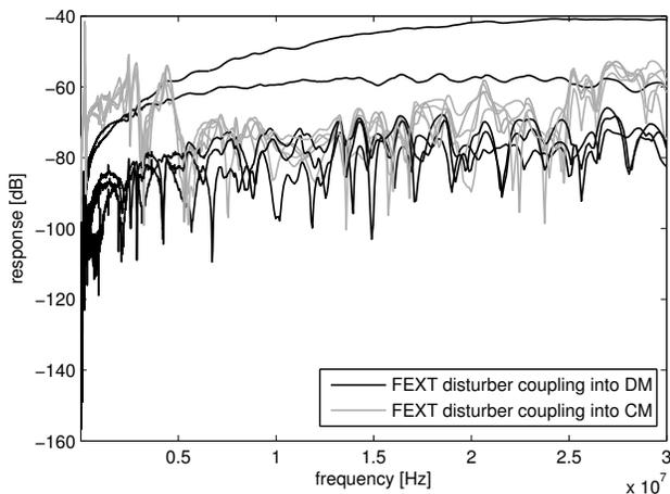
Fig. 4. FEXT coupling functions, obtained from measurements of different TPs in the bundle. The outliers are due to measuring adjacent TPs
