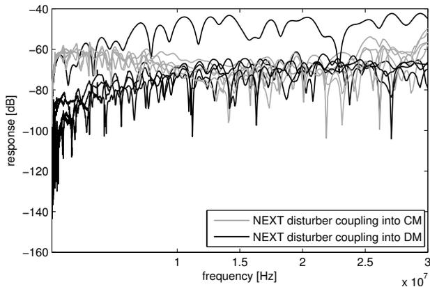
Fig. 3. NEXT coupling functions, obtained from measurements of different TPs in the bundle. The outlier is due to measuring the other TP in the same quad.
