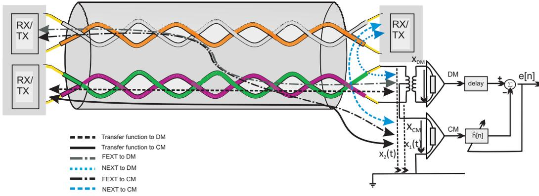
Fig. 1. Coupling functions and canceler structure
