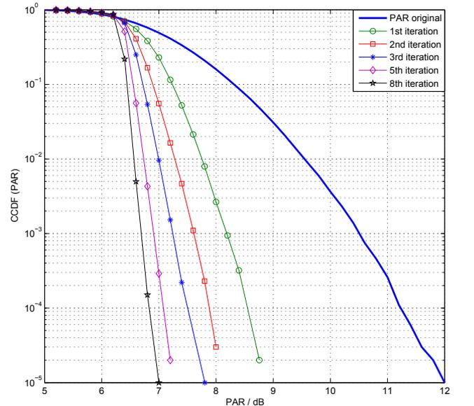
Fig. 4. CCDF(PAR) of the LS algorithm for a PAR target value of 6.5 dB without mean power constraints ( $\gamma = 30$ )
