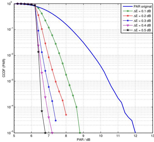
Fig. 7. CCDF(PAR) of the LS algorithm with a weighting factor  $\gamma = 30$ , for a PAR target value of 6.5 dB with different mean power constraints  $\Delta E$
