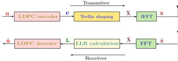
Fig. 2. Irregular LDPC code concatenated with Trellis Shaping
