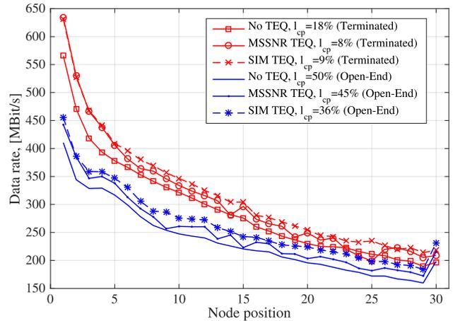
Fig. 6. Data rates in a 30-nodes bus system with constant CP, with and without termination, cable configuration  $l_R.l_M.l_B = 100.1.1$ ,  $N = 128$ .
