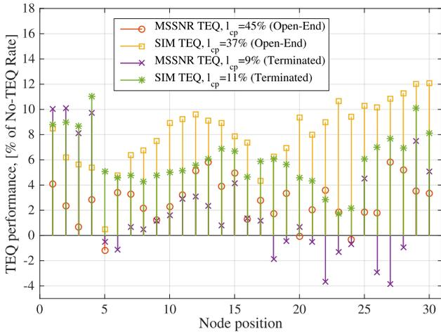
Fig. 7. Data rate gain with a TEQ compared to the corresponding data rate without TEQ in a 30-nodes bus system with constant CP, with and without termination, cable configuration  $l_R.l_M.l_B = 50.1.1$ ,  $N = 128$ .
