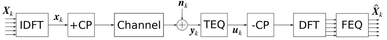
Fig. 1. DMT system with a time-domain equalizer (TEQ) at the receiver. The serial/parallel conversions are included in the DFT implementation (FFT).
