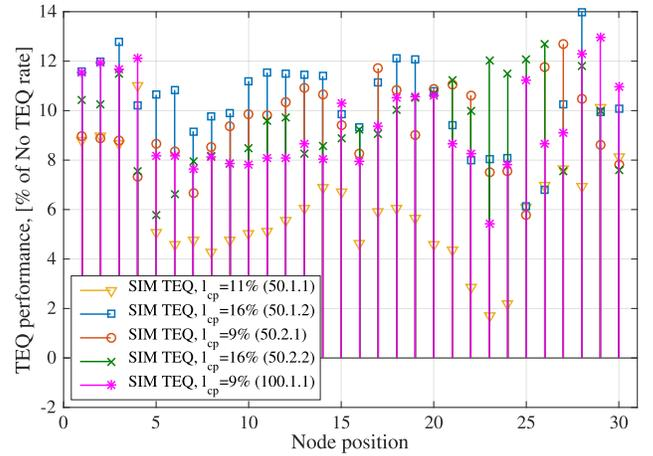
Fig. 10. Data rate gain of SIM-TEQ in a 30-nodes bus system with constant CP, with termination,  $N = 128$ .
