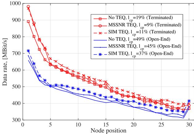
Fig. 4. Data rates in a 30-nodes bus system with constant CP, with and without termination, cable configuration  $l_R.l_M.l_B = 50.1.1$ ,  $N = 128$ .
