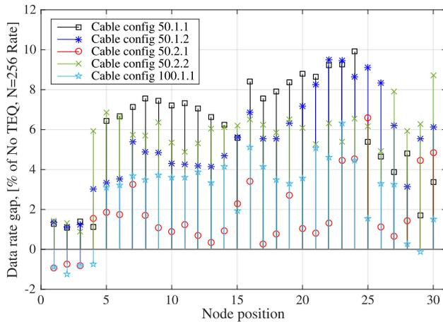
Fig. 11. Data rate gap between SIM-TEQ enabled system,  $N = 128$  and a system without TEQ and twice the FFT size (30-nodes bus system with constant CP, with termination).
