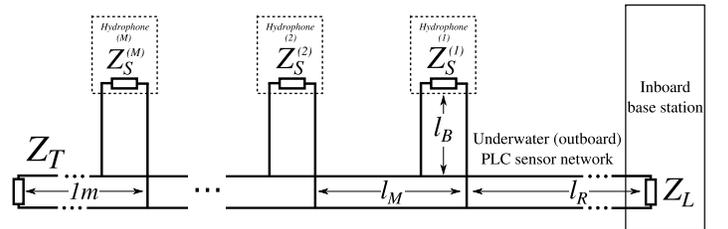
Fig. 2. An example bus system for simulations.
