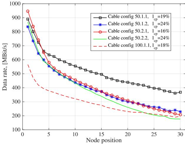
Fig. 8. Data rates in a 30-nodes bus system with constant CP, with termination, No TEQ,  $N = 128$ .
