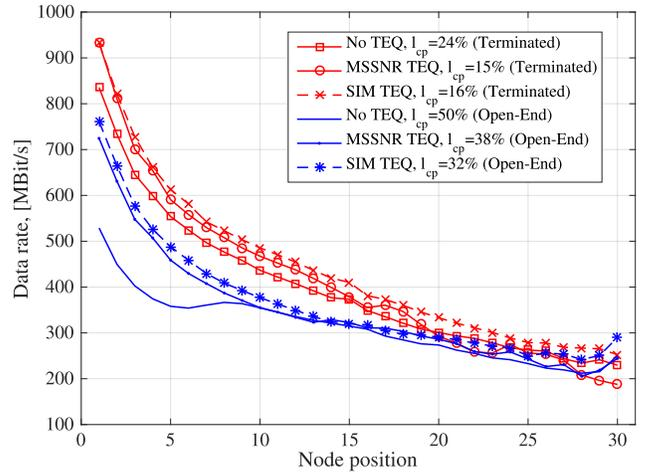
Fig. 5. Data rates in a 30-nodes bus system with constant CP, with and without termination, cable configuration  $l_R.l_M.l_B = 50.1.2$ ,  $N = 128$ .
