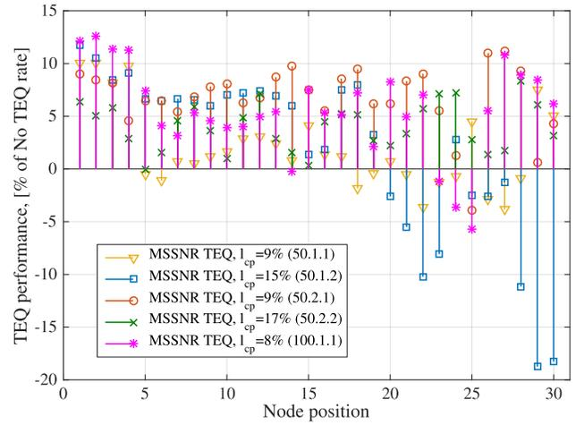
Fig. 9. Data rate gain of MSSNR-TEQ in a 30-nodes bus system with constant CP, with termination,  $N = 128$ .
