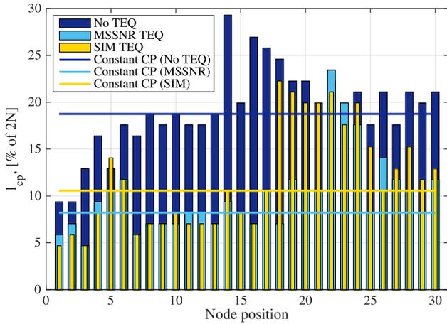
Fig. 3. Estimated optimum cyclic prefix lengths in a 30-nodes bus system, cable configuration  $l_R.l_M.l_B = 50.1.1$ ,  $N = 128$ .
